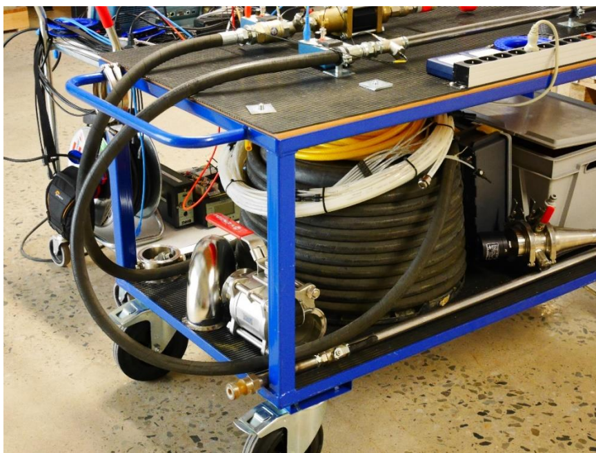
Figur 90. 20 m hoprullad injekteringsslang. Coiled rubber tube on lower shelf.
